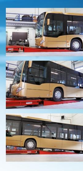
In doing so, vehicle configurations of up to 30 metres in length and with a total weight of up to 70 tonnes can easily be lifted! The SKYLIFT is even flexible with regard to its width. During installation, the width between the platforms can be adjusted to the fleet of vehicles.
